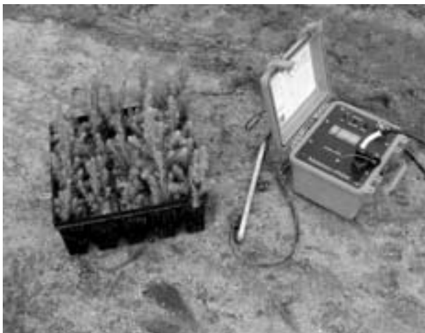
Figure 1. Determination of substrate water content in an IPL-25-350A seedling container using the MP-917 soil moisture system.
