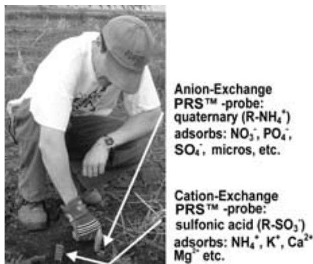
Figure 2. PRS™-probes used to measure soil nutrient availability in situ .
