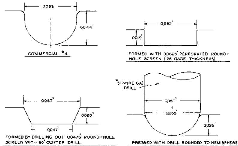
Figure 11. Indents used for removing pigweed from alfalfa.
