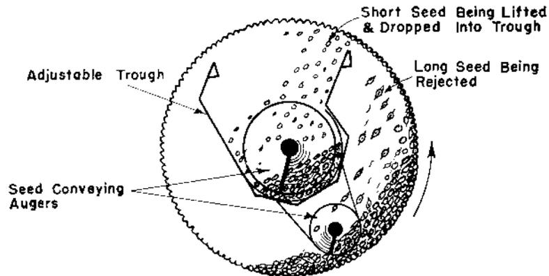
Figure 1. Cross-section view of an indent cylinder separator.
