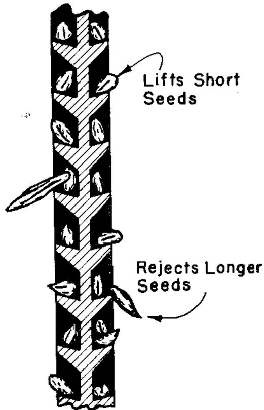
Figure 2. Cross-section view of an indent disc separator.
