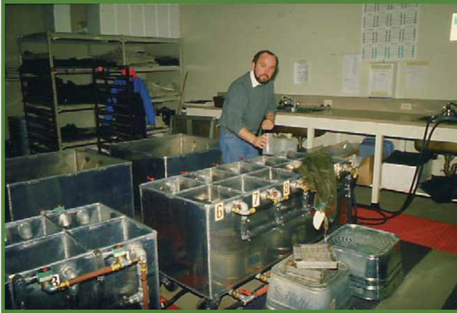
Figure 78 A large single- and a multi-chamber soaking tank used operationally at the BC Ministry of Forests Tree Seed Centre.
