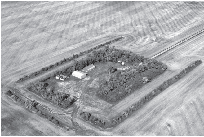
Figure 1. Eco-Buffers, consisting of long-lived and short-lived trees along with small, medium and tall shrubs are structurally complex compared to traditional, multi-row shelterbelt designs.
