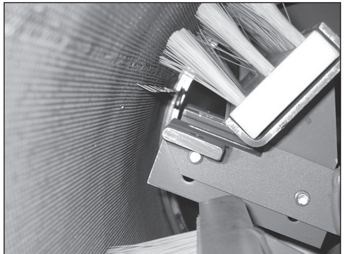
Figure 5. Brush-cleaning combs keep awns from clogging rotating brushes in a Westrup HA-400 (Huntsman, Incorporated, Twin Falls, ID).
