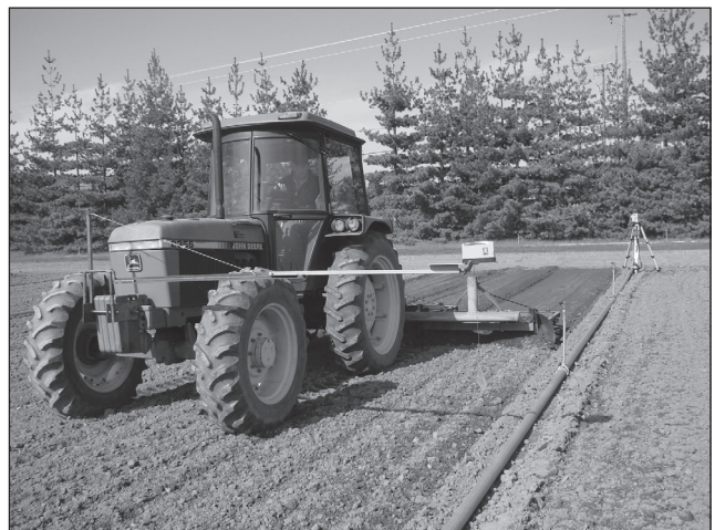
Figure 12. A rotary laser, used vertically, projects a beam of light to help field personnel lay out irrigation pipelines and nursery beds in a straight line.
