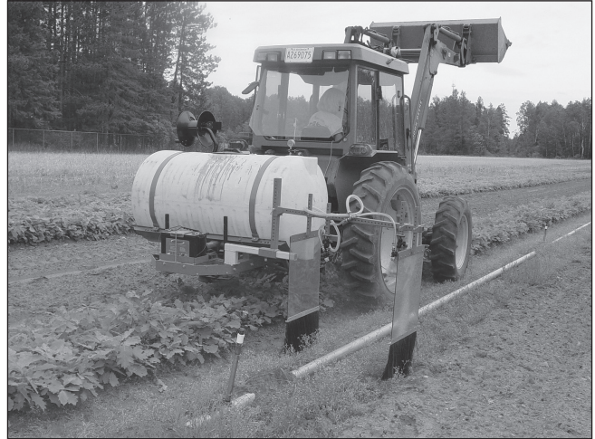
Figure 11. A sprayer shield assembly is shown mounted to a three-point hitch sprayer designed specifically for spraying around irrigation pipelines.
