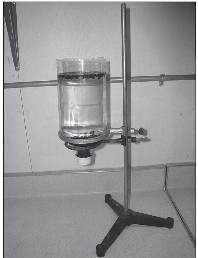
Figure 7. A large plastic soda bottle can be used to separate seeds in the Imbibe, Dry, Separate (IDS) procedure.
