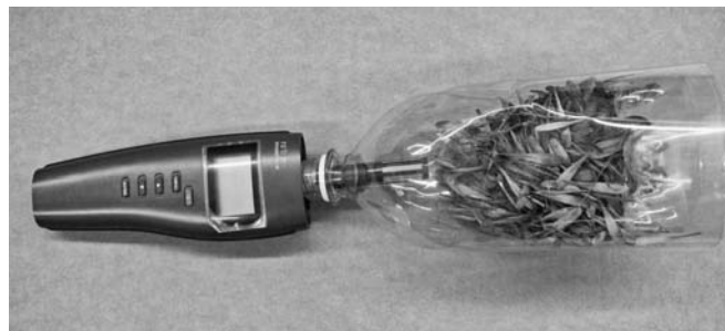
Figure 5. A 2-L (0.5-gal) plastic drink bottle converted to a chamber to measure ERH with a hygrometer.
