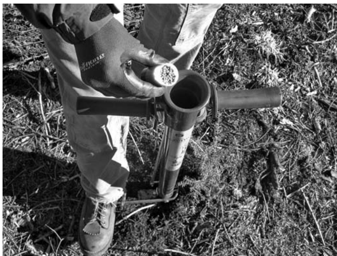
Figure 1. Pottiputki planting tool used to deliver controlled-release fertilizer 5 cm (2 in) uphill of the seedling and 5 cm (2 in) below the soil surface.
