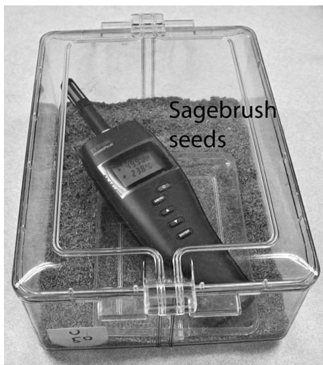
Figure 4. Measuring the ERH of sagebrush seeds by placing the hygrometer (Rotronic Instruments USA, Huntington, NY) entirely inside a plastic box containing the seeds.
