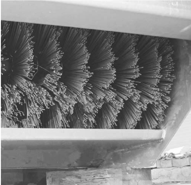
Figure 4 —Stiff bristles with convoluted wafers worked better than the factory brushes to collect small forbs seeds on this Woodward Flail-Vac Seed Stripper.
