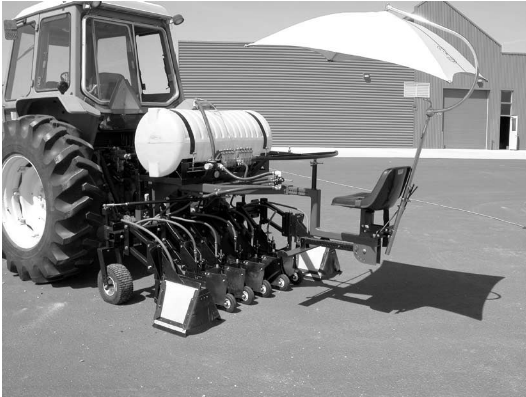
Figure 2—MTDC's improved shielded herbicide sprayer was evaluated in Virginia.
