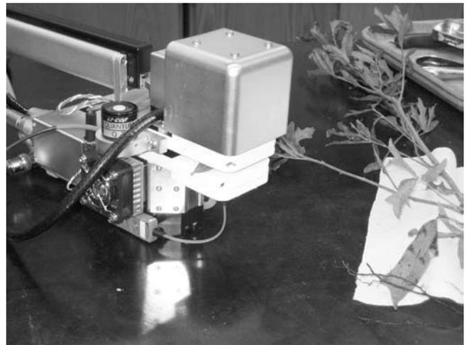
**Figure 1**—Detached leaf in leaf chamber for chlorophyll fluorescence and net photosynthesis measurements using an open gas exchange system (LI-6400; LI-COR Inc., Lincoln, NE) with an integrated fluorescence chamber head (LI-6400-40 leaf chamber fluorometer; LI-COR Inc.).
