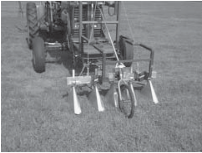
Figure 1 —A directed herbicide sprayer for hardwood seedlings at the East Tennessee Nursery.
