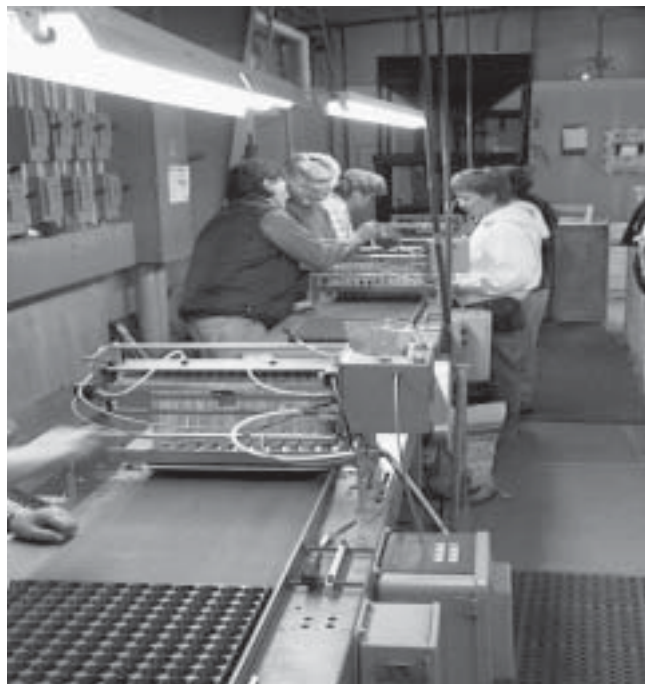
Figure 10—Container seed drill with double heads for addition of slow release fertilizer to cells.
