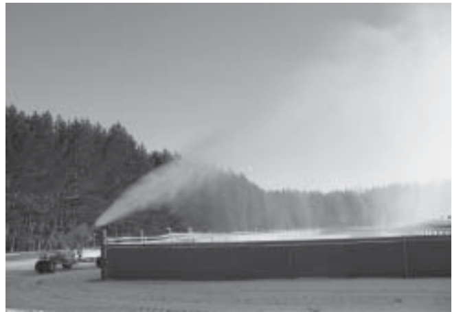
Figure 13 —Snowmaking equipment for overwintering seedlings.
