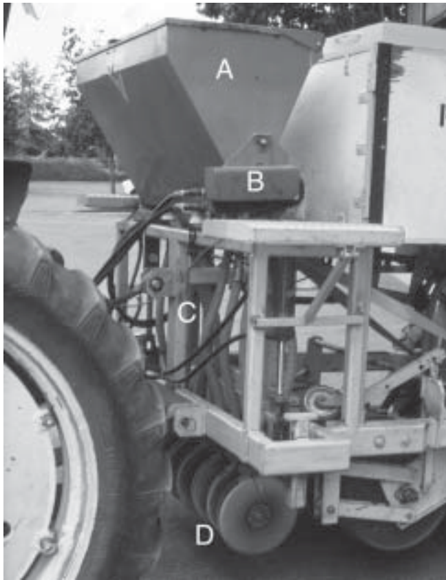
Figure 2 —Bander consists of fertilizer hopper (A), hydraulically controlled, chain-driven fertilizer meter (B), drop tubes (C), and coulters (D) that place fertilizer in the soil.
