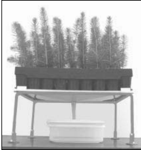
Figure 2. Leachate collector with plate and vessel. One-year old Norway spruce seedlings in Plantek 81F container tray. (Photographed by Pekka Voipio)
