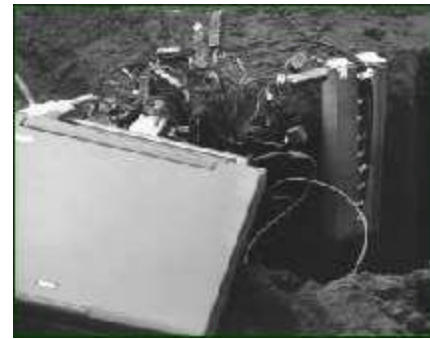
Figure 12. The thermocouple array used to determine the vertical soil temperature profile. A pit was dug for the instrument immediately after steam treatment.
