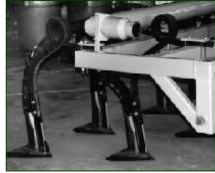
Figure 5. Sweeps (triangular plates) helped the shanks distribute the steam more evenly than when the vertical shanks were used.
