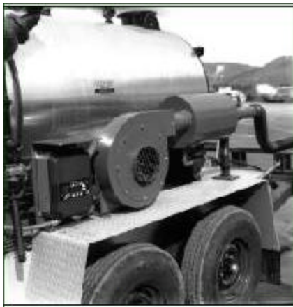
Figure 2. The electric blower adds air to regulate the temperature of the steam.
