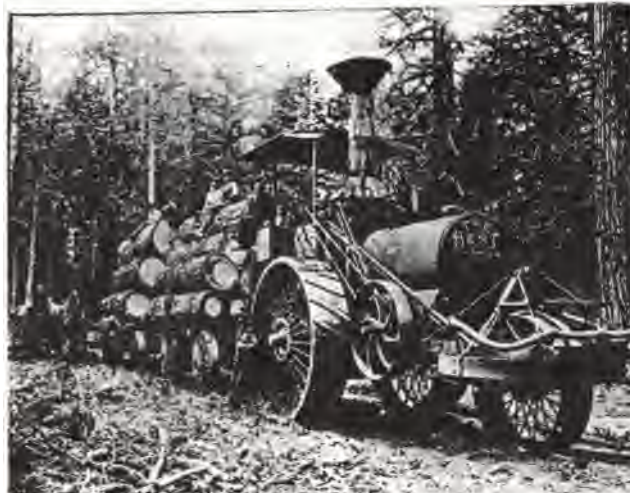
C. L. Best Steam Tractor (vertical fire tube boiler), 1885.
