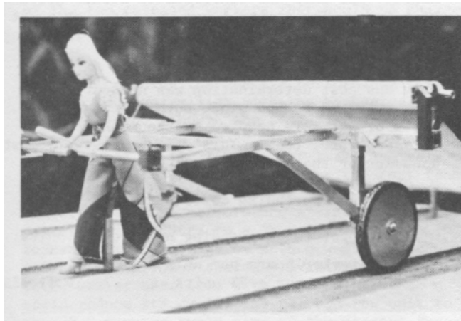
Figure 3.--An Oregon State University model was the pattern for building the labor saving cart to assist workers placing new or precut net over seeded bed-rows.
