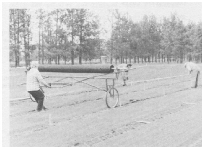
Figure 4.--During testing one worker guides the cart along the bed while two workers stretch and hook the net to stakes.
