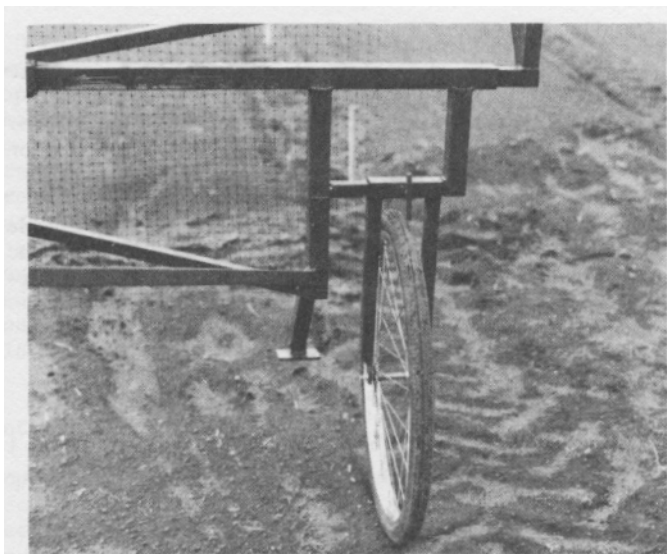
Figure 5.--There are several adjustable components on the machine. The one shown permits change in the distance between wheels to fit variations in bed width.
