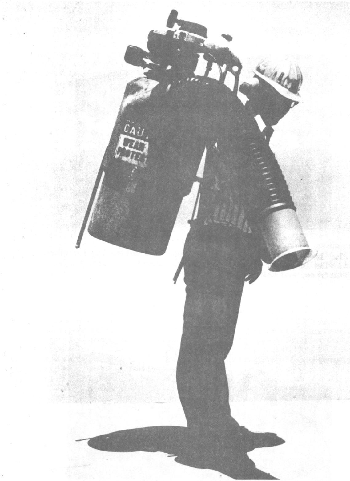
Fig. 3. Experimental model of a back-pack seed harvester used in obtaining seed from a variety of shrubs. This equipment is most effective for plumed seeds.
