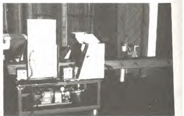
Figure 11.--View of seeder, gritter, conveyor and support frame assembly.
