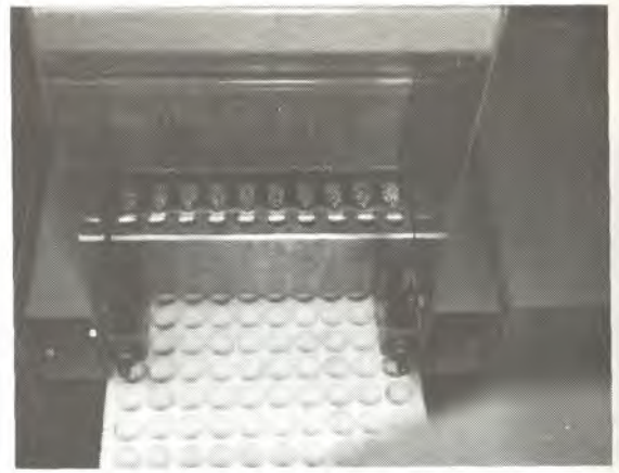
Figure 10.--Seed covering machine hopper assembly.
