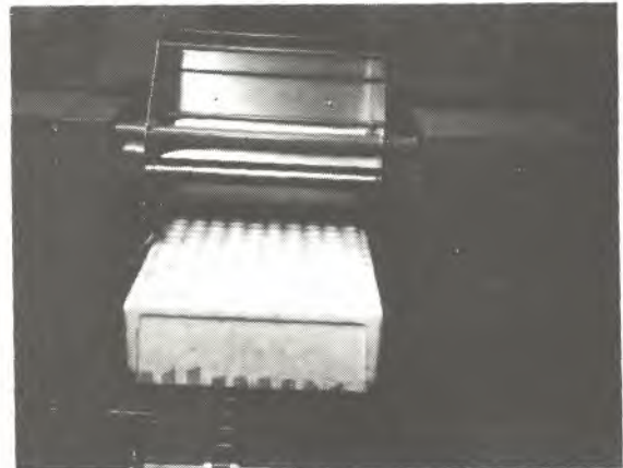
Figure 7.--View of seeder and conveyor assembly.
