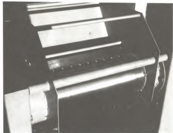
Figure 5.--View of seed drum and air brush.
