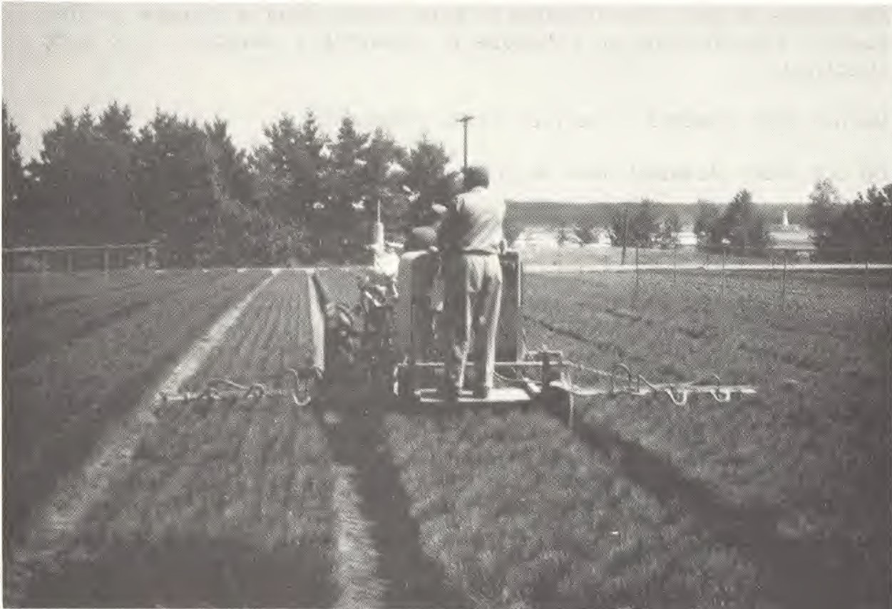
Figure 4. - A hydraulic sprayer used by a Wisconsin Nursery to apply Maneb to red pine nursery beds for Lophodermium control. Hugo Sauer Nursery, Rhineland, Wisconsin
