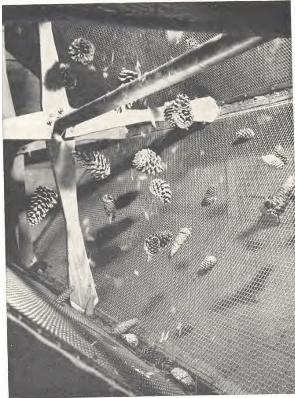
FIGURE 16.—Interior of power-driven progressive cone tumbler, viewed from large end. For specifications write Regional Forester, U. S. Forest Service, Atlanta, Ga. (Photo courtesy of Louisiana Forestry Commission.)
