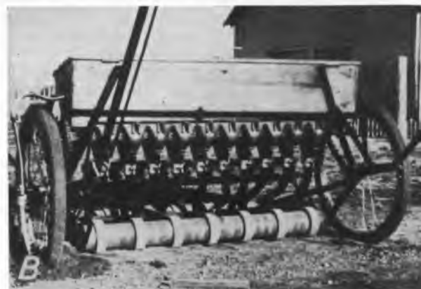
FIGURE 13.—A, Standard 4-foot-wide, 10-row conifer seed drill. Seeding rate can be adjusted by changing the size of the sprocket gears on the right side of the machine. The machine is pulled by two men or by a bed-straddling tractor. B, A 7-row seed drill with flanged roller that controls depth of seeding.
