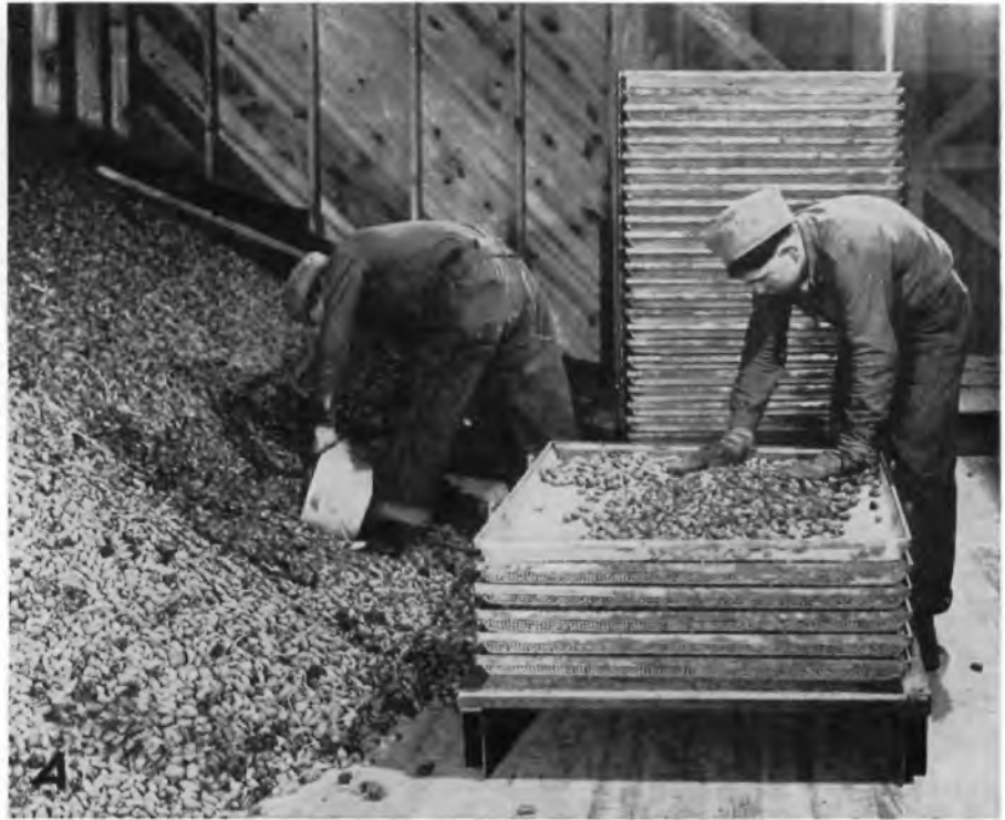
FIGURE 2.—A, Loading kiln trays with cones. B, Two-unit cone kiln designed by U. S. Forest Products Laboratory. (Chittenden Nursery, Wellston, Mich.)
