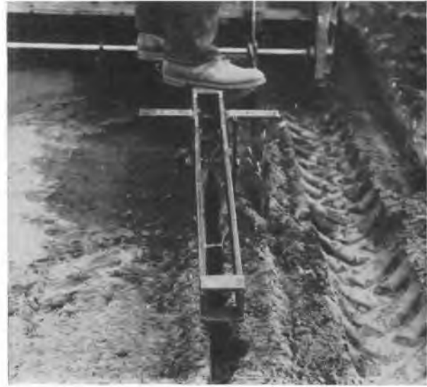
FIGURE 47.—A tractor-drawn trencher in position. Operator rides this trencher to control depth and aid in steering.
