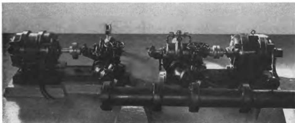
FIGURE 8.—Pump on right is a 225-gallon-per-minute, double-suction centrifugal, driven by a 15-hp., single-phase, electric motor. Pump on the left is of the same type and capacity but made by a different manufacturer.
