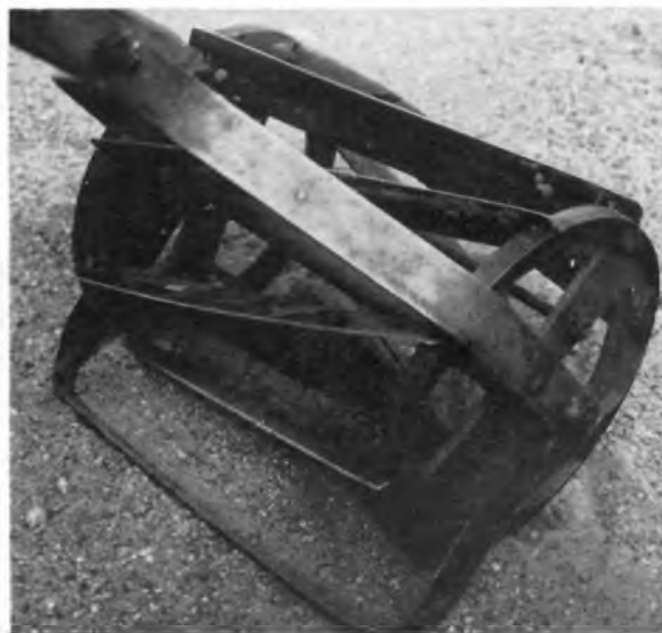
FIGURE 21.—A 10-inch-wide rotary hand weeder suitable for weeding paths and rows of broadleaves or transplants at 12- to 14-inch spacing in sandy nursery soils. The blade at the lower left cuts weed roots horizontally and the angled blades on the revolving reel pulverize the soil.
