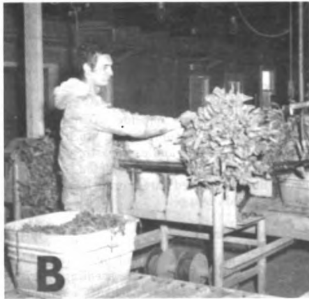
Figure 49.—Baling European alder seedlings at the Illinois Mason State Nursery: A, Belt-type baler operated by electric hoist; B, forming a veneer-mat bale.
