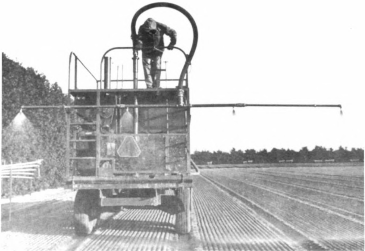
Figure 27.—The hydromulcher sprays wood fiber onto the seedbed in a water slurry. (Photo courtesy Saratoga Nursery, New York State Conservation Department.)
