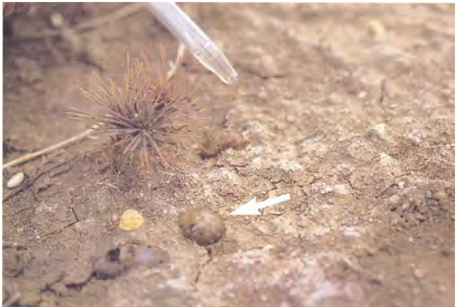
Figure 31-3. The presence of excessive calcium salts can be confirmed by placing a drop of dilute acid on the soil to see if effervescence occurs.
