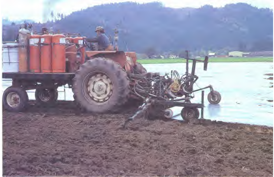
Figure 33-10. Methyl bromide-chloropicrin fumigation is commonly used to decrease populations of nursery pests in the soil. Chemical is injected into the soil and then a tarp is laid to trap the gas.
