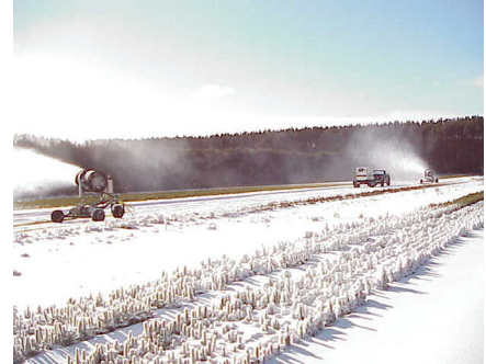
Figure 54.9 —Snow blowers are used in Northern States to coat seedlings in snow for protection from winter burns. Photo from Minnesota Department of Natural Resources.
