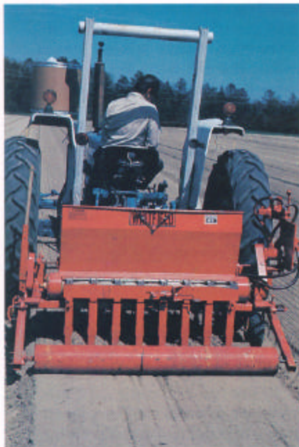
Figure I-11 —Machine for applying mycelial inoculum to nursery beds.
