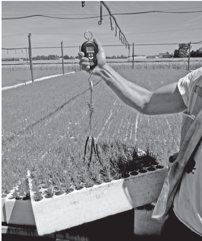
Figure 2 - A Styroblock® container fitted with basket hangers has its weight measured with an inexpensive, portable, hand-held, digital balance (Dumroese and others 2015).
