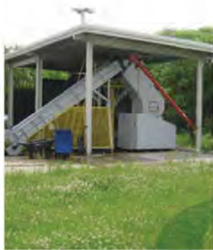
The Garden purchased a granulator and conveyor to process plastic into chips.
