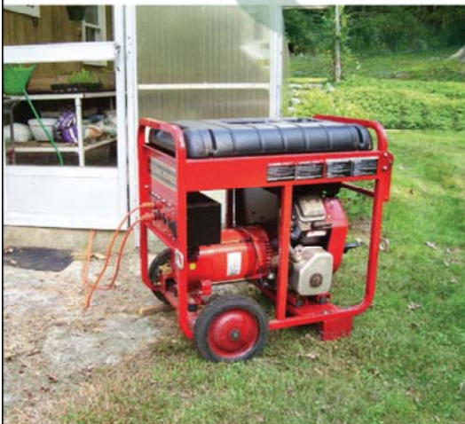
Engine-driven units can be powered by gasoline, LP gas or diesel fuel.
