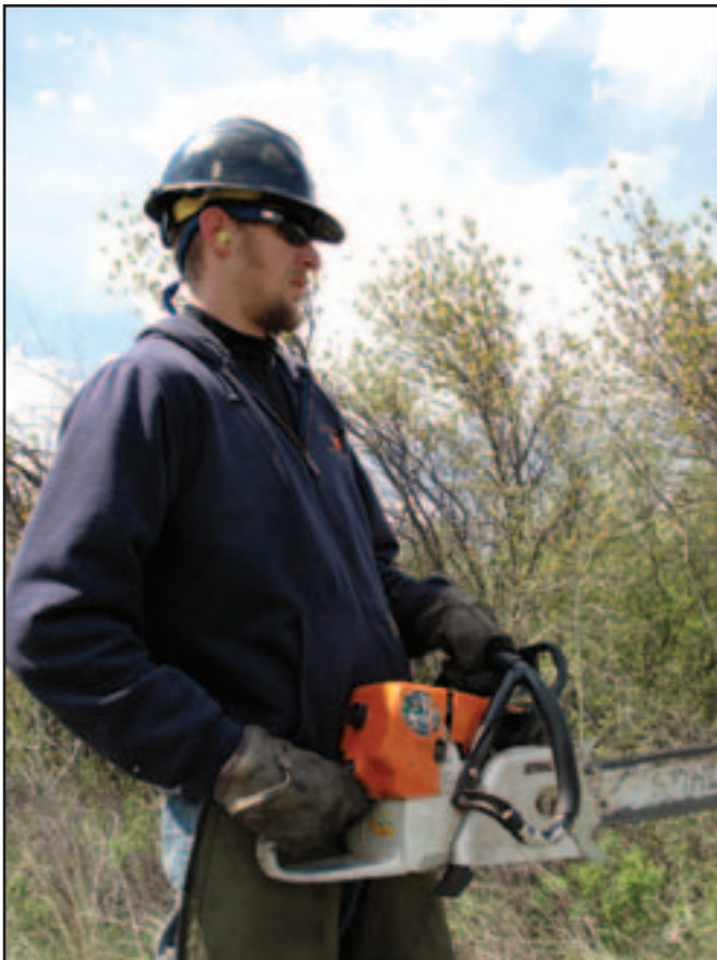
Figure 1—Hearing protection devices, such as earplugs, must be worn while operating a chain saw. Noise from the saw will vary depending on the angle of the saw.
