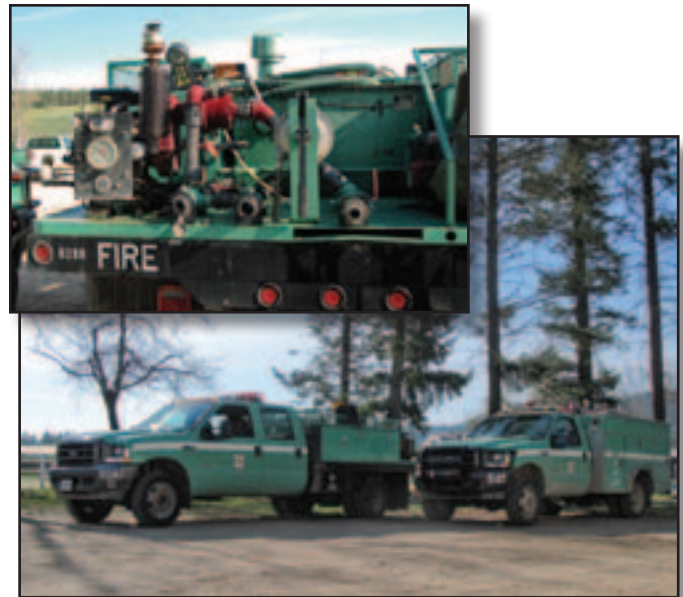
Figure 2—Most firefighters know that noise from equipment can compromise their hearing. The noise level of a pumper engine (inset) is 94 to 97 dB. They may not know just driving to the worksite with the vehicle's windows down also can cause harm.
