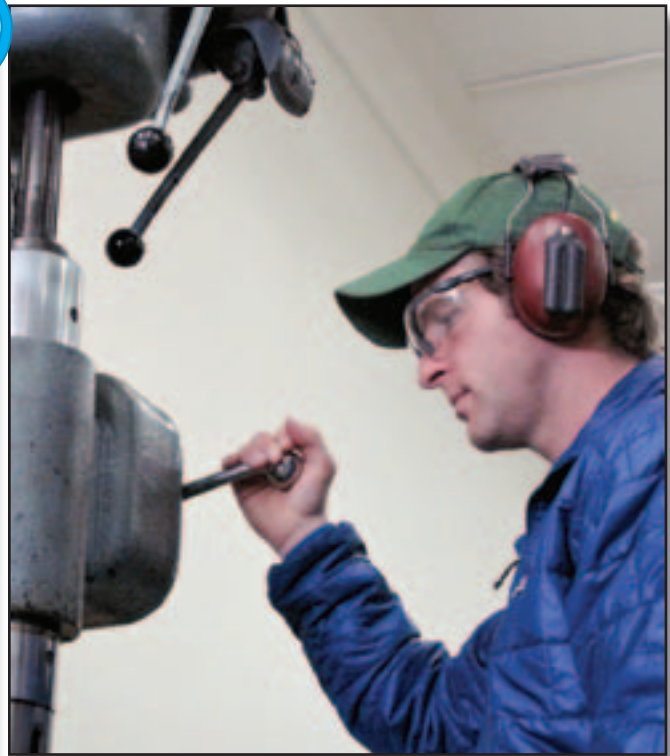
Figure 13—Ear muffs are often the preferred type of hearing protection in shop settings.
