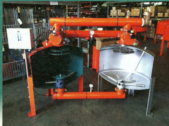
Filters composed of stainless and carbon steel—and illustrated in Figures 1 and 2—are cut away to show the inner workings.
