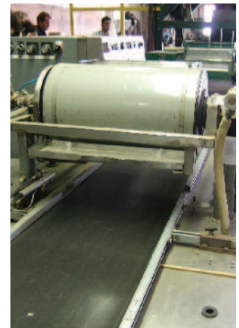
VACUUM DRUM SEEDER – SINGLE REVOLUTION PER COPPERBLOCK
