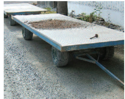
PNEUMATIC TIRED TRAILERS, HOLD 100 COPPERBLOCK TRAYS EACH.
