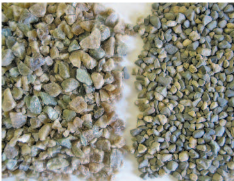
STYROGRIT (LEFT) – FRASER RIVER GRANITE GRIT (RIGHT)
