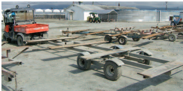
CUSTOM BUILT TRAILERS FOR MOVING COPPERBLOCKS TRAYS ON CUSTOM PALLETS
