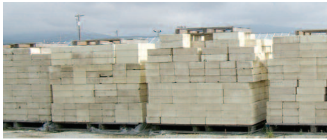
COPPERBLOCK STORAGE – NOTE PALLET ON TOP.
