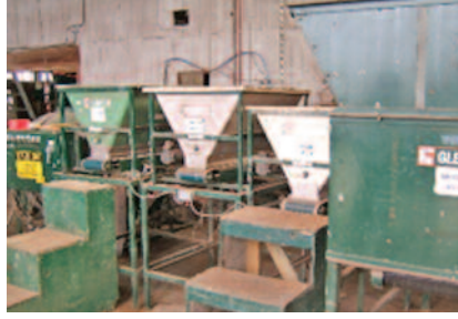
CONTINUOUS MIXING LINE – DRUM MIXER TO THE LEFT.
