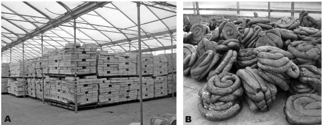
Figure 1 – Many nurseries are plagued by stacks of used Styroblock™ and Copperblock™ containers, that cannot be recycled or taken to landfills (A). A new process grinds and compresses the used blocks into a more easily disposable product (B).
