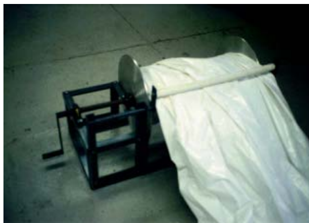
Hand reel for rolling plastic has tapered core and removable end plate.
