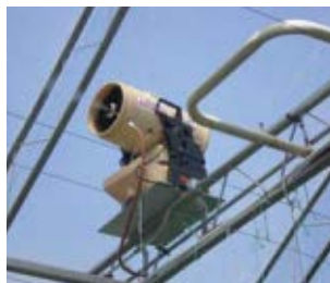
TOP: Because of a Coldfogger's forceful, directed spray, it is often better at reaching deep into heavy plant canopies.
