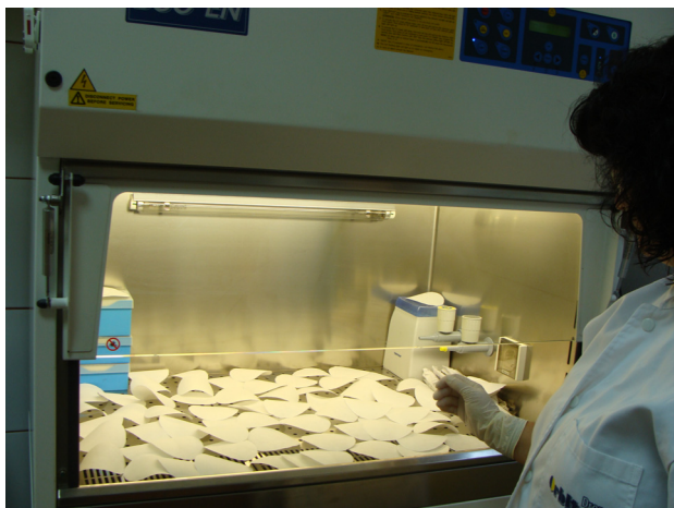
Figure 2. UV sterilization of filter paper for seeds germination samples
