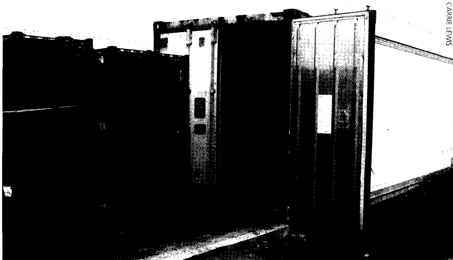
Heritage Seedlings has modified this insulated shipping container to use it as a chamber for pasteurizing used containers and propagation flats.
