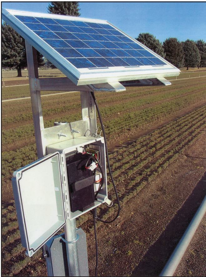
Figure 6—The solar panel's power box opened to show the gel cell battery and voltage regulator.
