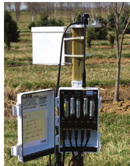
A Decagon Devices Inc. EM50R node is connected to a tipping rain gauge, light (photosynthetically active radiation) sensor and three soil-moisture sensors (not visible) in the field.
