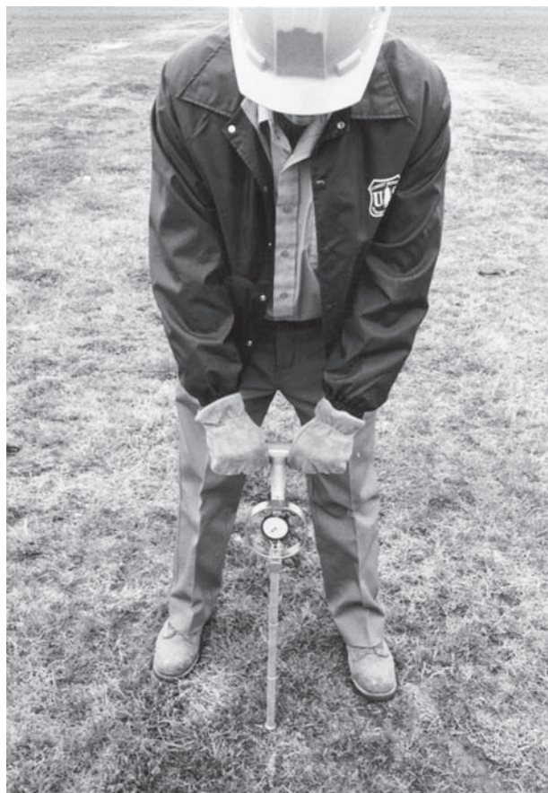
Figure 3.3. Soil penetrometer being used to assess soil compaction.
