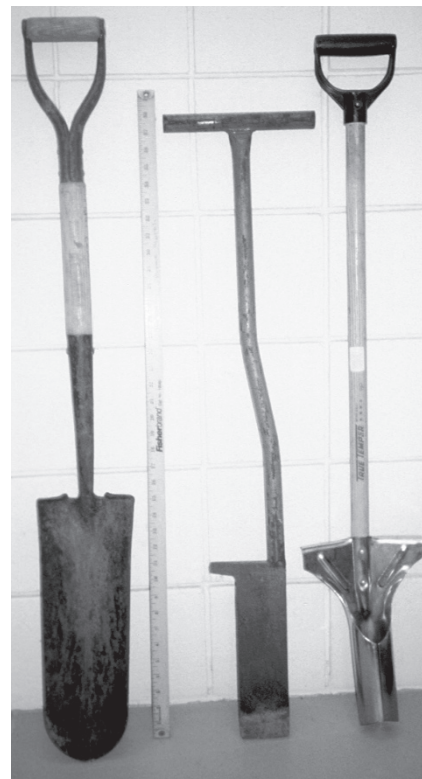
Figure 8.8. Bare-root seedlings can be planted using a sharpshooter shovel, dibble bar, or bulb planter.
