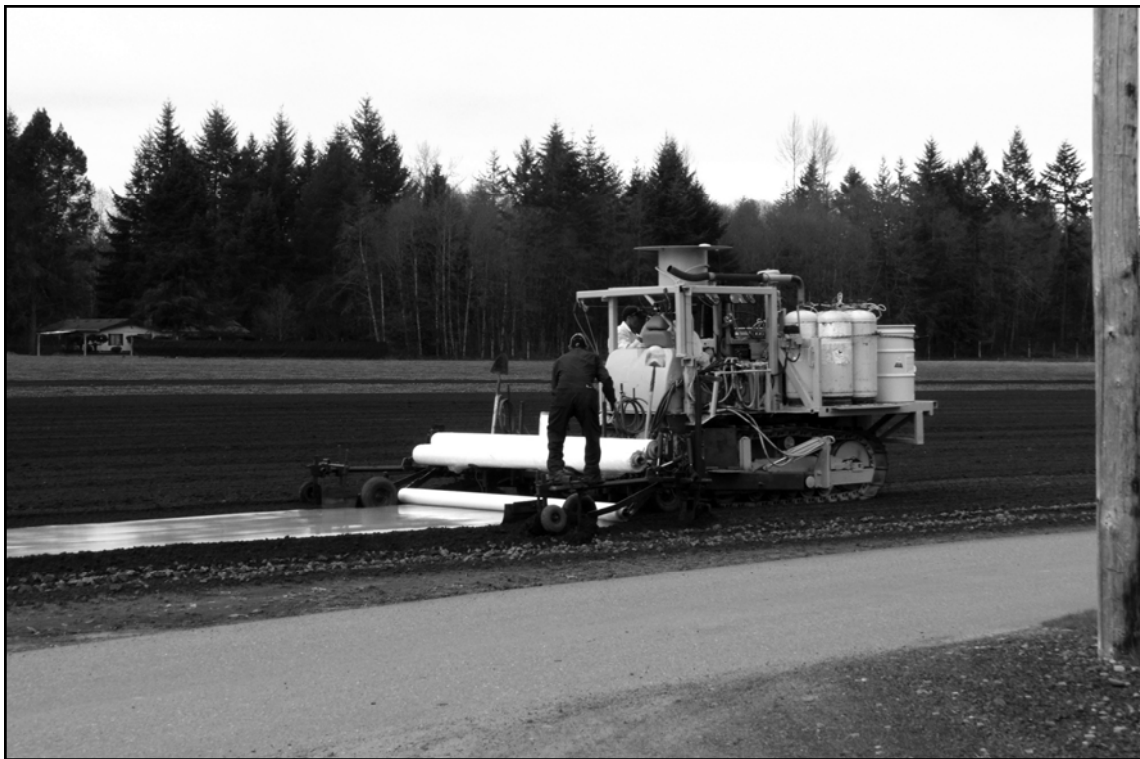
As methyl bromide is injected into the soil, it is immediately covered with a plastic tarp
