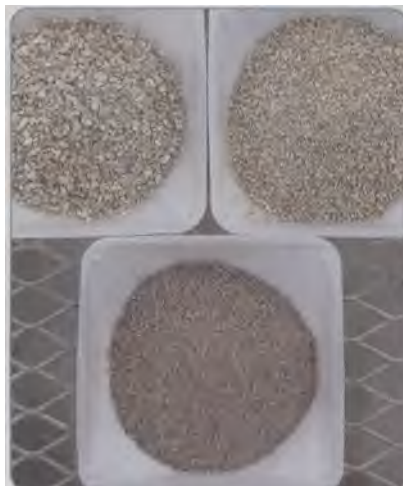
Vermiculite comes in different size grades, which affects its physical properties. The source of the ore used to make vermiculite can have a significant effect on its chemical properties.
