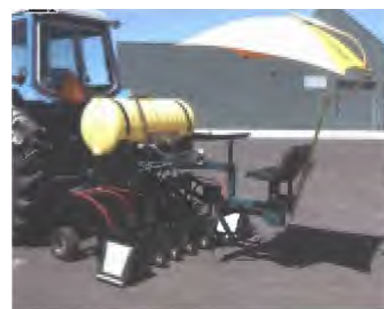
Figure 7. The MTDC shielded herbicide sprayer has adjustable spray hoods and a tiller steering system.
