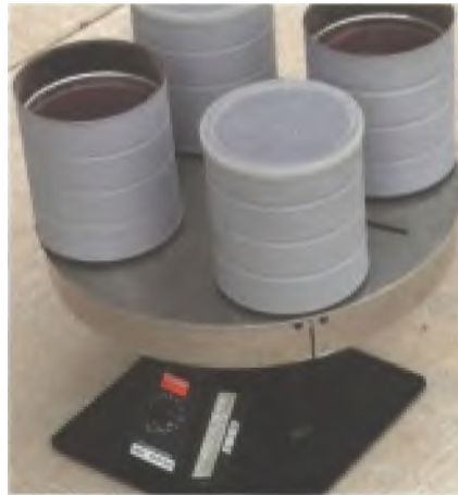
Figure 7. Seeds in the whitebark pine seed scarifier swirl across sandpaper that lines each of the four cans.
