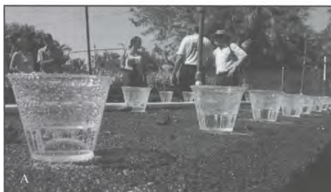
Figure 2—The best way to test irrigation sprinkler efficiency is the "cup test" (A), a regular grid where the depths or volumes of water are measured at each point (B). Photo A by Kim Wilkinson
