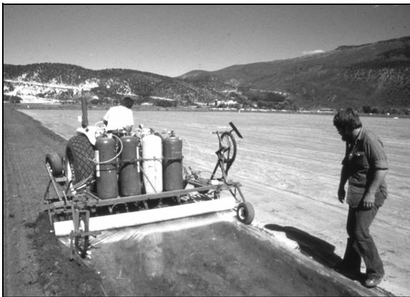
Figure 1—Plastic tarping is standard practice for methyl bromide/chloropicrin fumigation, whereas dazomet and meta-sodium fumigants are contained with a roller and water seal.
