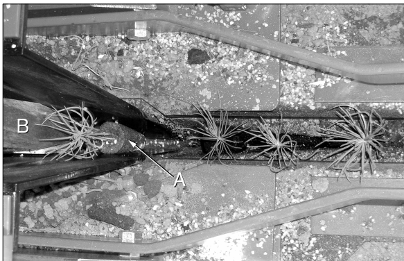
Figure 3. As transplanter moves to the left, a Q-plug drops into the soil (A) and is placed into an upright position with a moving paddle (B). The soil furrow is immediately closed.
