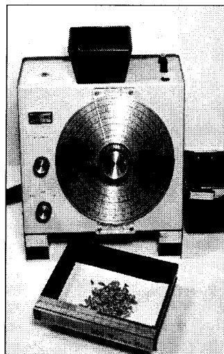
Figure 8. Because it is so critical to maintaining viability during storage, nurseries should monitor seed moisture with electronic meters, such as this Dole/Eaton Model 400 (Courtesy of Agri-Tronix Corporation).
