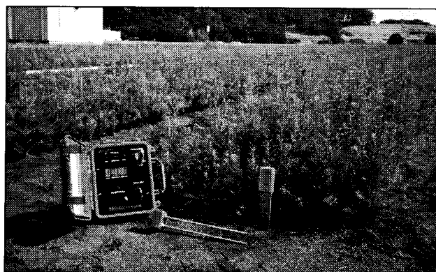
Equip 11A. Moisture-Point TDR™ meters give a digital readout of % moisture using probes that are designed for bareroot nursery soils. (Courtesy of Environmental Sensors, Inc.)
