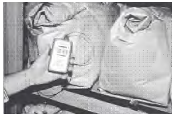
Figure 3. Although ambient temperature readings indicate how the refrigeration equipment is functioning, the true indication of storage temperature can only be obtained with in-bag monitoring.
